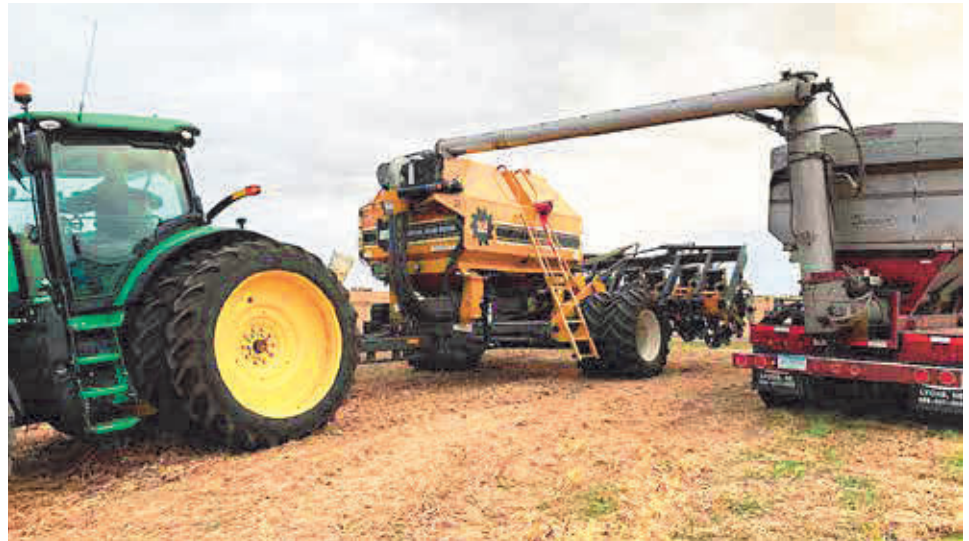
The Wilts' family uses an Environmental Tillage System Soil Warrior for strip tillage and fertilizer application in the fall.
